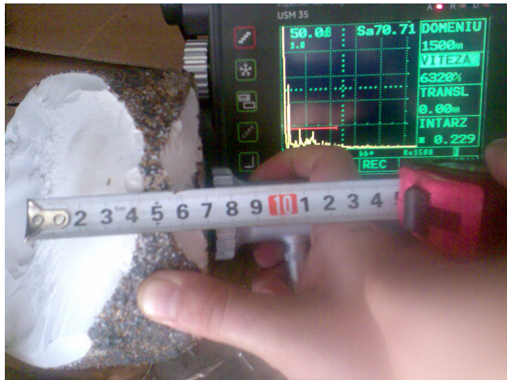
Fig. 2.5. Confirmation of the discontinuity indication at 70 mm.
